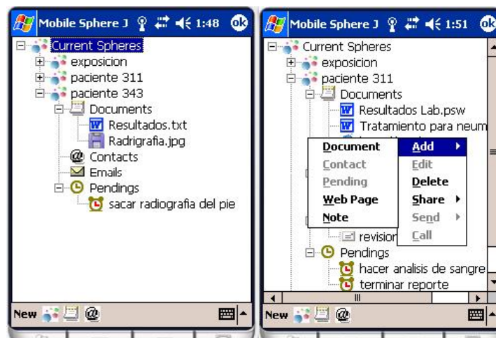
Fig. 7. Interface of the mobileSJ. Different types of resources, such as documents, contacts and pending tasks can be associated to working spheres and then manipulated from the application
