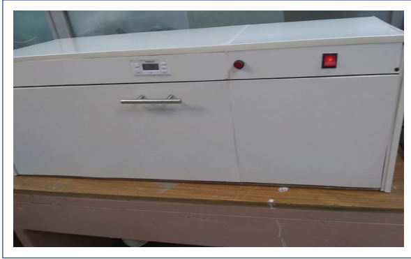
Figure 8. An ultraviolet lightbox designed by the Biomedical Engineering department to re-sterilize N95 respirators. It contains two 280 nm lamps that emit radiation in the range of 280-420 nm to achieve exposure of 0.5-1 J/cm 2 .
