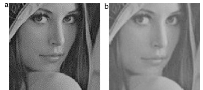
Fig. 6. (100 × 100) grayscale image: (a) in a traditional pixel format and (b) in a piecewise-linear function interpolated format.
