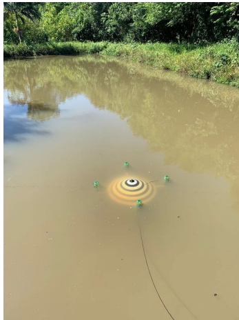
Figure 4. Reference cone for aerial images, for the purpose of analysis of the bodies of water transparency in a fish farming environment.
