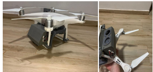
Figure 3. Equipment for image capture of fishponds attached to an RPAS (prototype).
