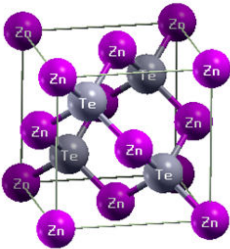
FIGURE 1. Blende structure ZnTe.
