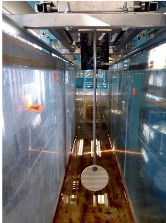
Figure 8. Device to measure the hydrodynamic thrust on a porous disc.
